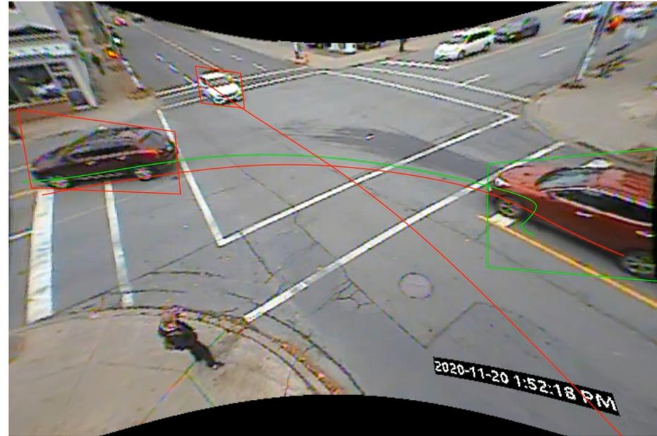
North-left vs South-through: PET = 2.5s, vehicle speed 52 km/h
