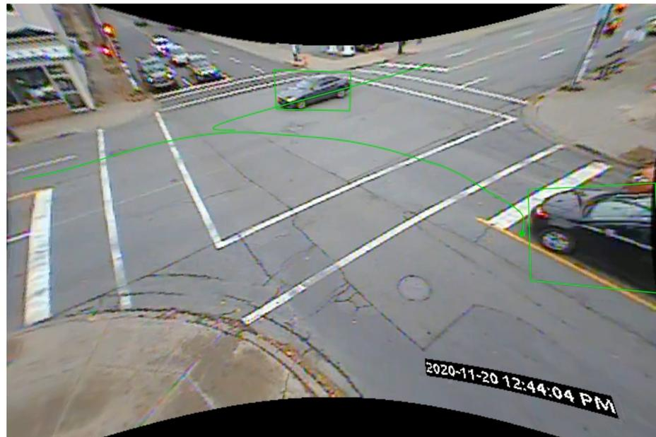
East-through vs North-through: PET = 2.8s, vehicle speed 20 km/h
