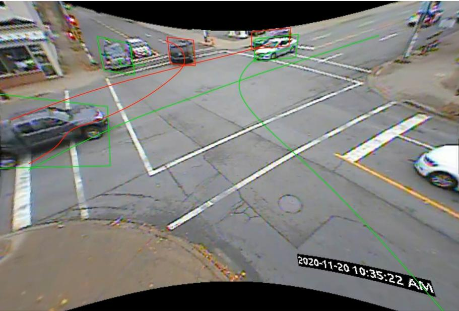
East-left vs West-through: PET = 1.8, vehicle speed 36 km/h
