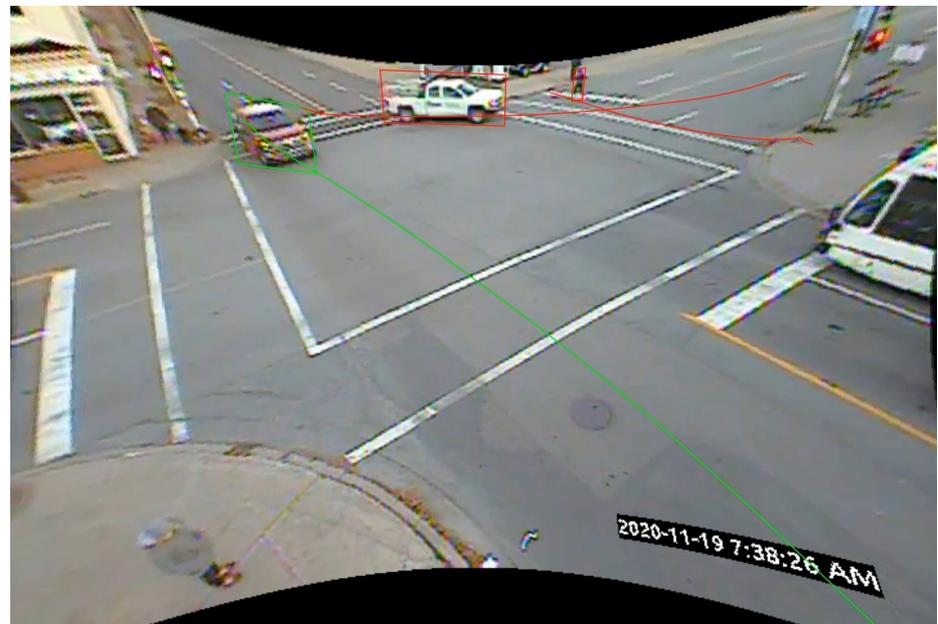
Pedestrian South-Left Hook:  $T_2 = 1.9s$ , vehicle speed 23 km/h
