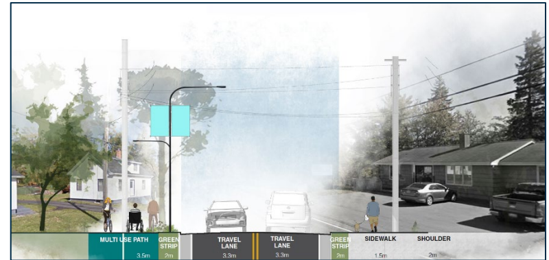
Example of a sidewalk and multi-use pathway on Trunk 3 in Hubbards
