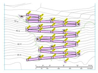
**Schematic 2** shows a ramp system made of 30 ramp segments with landings, each ramp section is 9m run x 0.6m rise and has handrails. There are 8 rest stops with benches along the route spaced out on every third to fifth landing (approx. 30 to 50m). The intent would be to build the ramp system into the hill matching closely with existing grades.
