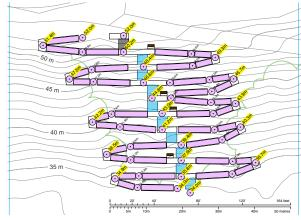
**Schematic 3** shows the incorporation of staircases with the ramps. There is a rest stop with a bench on every second or third landing. The benches provide places to sit with scenic views out to the lake. While this option has the most infrastructure, it provides the best option for accessibility providing both ramps and stairs.
