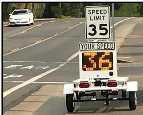
Most motorists are familiar with what are commonly referred to as 'speed reader boards' which are deployed roadside. The trailers have a front facing radar which detects and posts the speed of passing vehicles as well as the posted speed. Speed enforcement trailers have an additional rear facing radar which detects the speed of the vehicle once it has passed the trailer. If the vehicle is travelling above the threshold speed, the event is captured for image review and offence processing.
