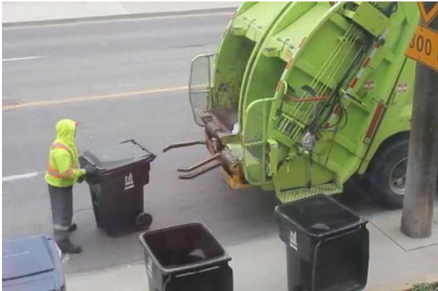
Figure 2: Semi-automated collection using a hydraulic tipper on the back of the truck.
