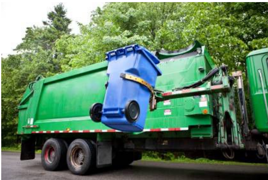
Figure 3: Fully-automated collection. Operator does not leave the cab of the truck.
