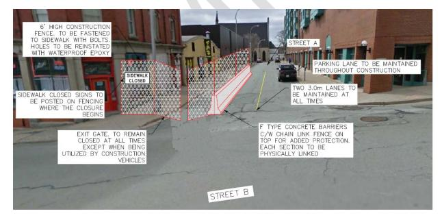
Figure 1 – Proposed delineated vehicle staging and delivery area; Street A. The Sidewalk is to be closed along this portion of the site; pedestrians must use the sidewalk on the other side of Street A.
