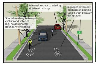
Figure 1: Typical Local Street Bikeway Cross Section
