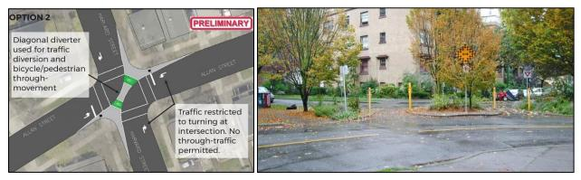
Figure 6: Plan View of Diagonal Diverter
