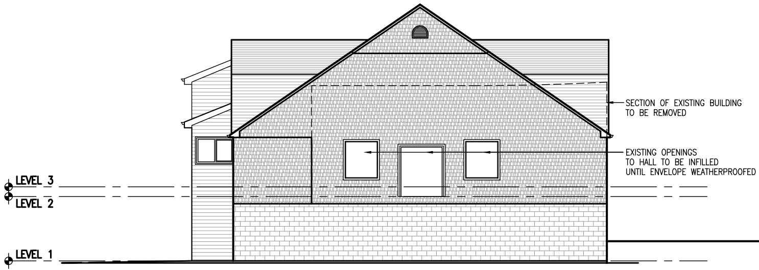
NORTH ELEVATION, POST PHASE 1 DEMOLITION
