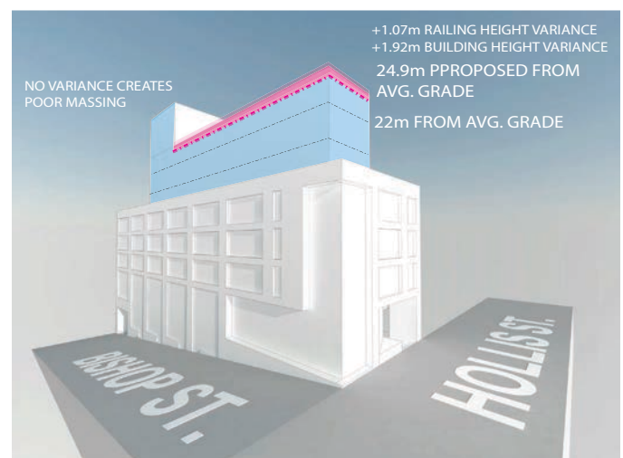
Figure 43. 22m Building Height from Average Grade
