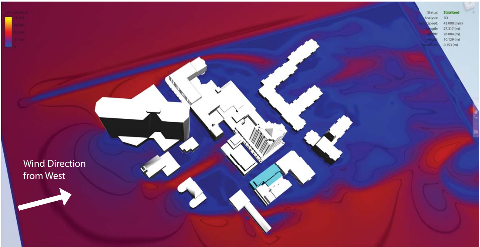
Fig 7. Westerley wind directions with starting wind speed at 30 m/s. Blue shows areas of calm (<30 m/s), while orange and yellow shows areas of increased wind speed (>30 m/s).
