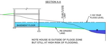
Figure 4-3: Incorporation of Elevation in Flood Mapping
