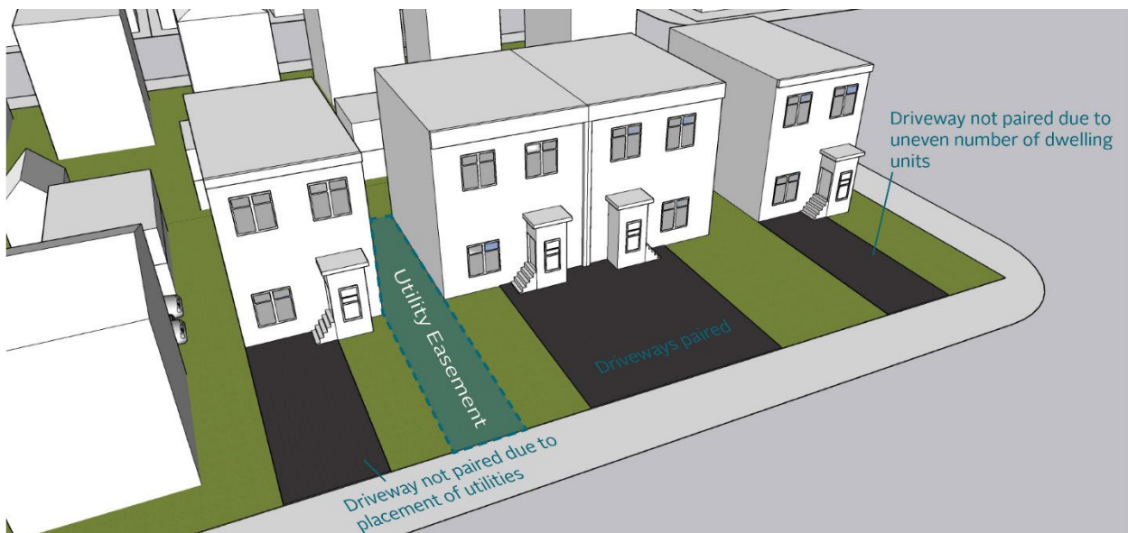
Diagram PG-7: Driveway pairing, per Section PG-127
