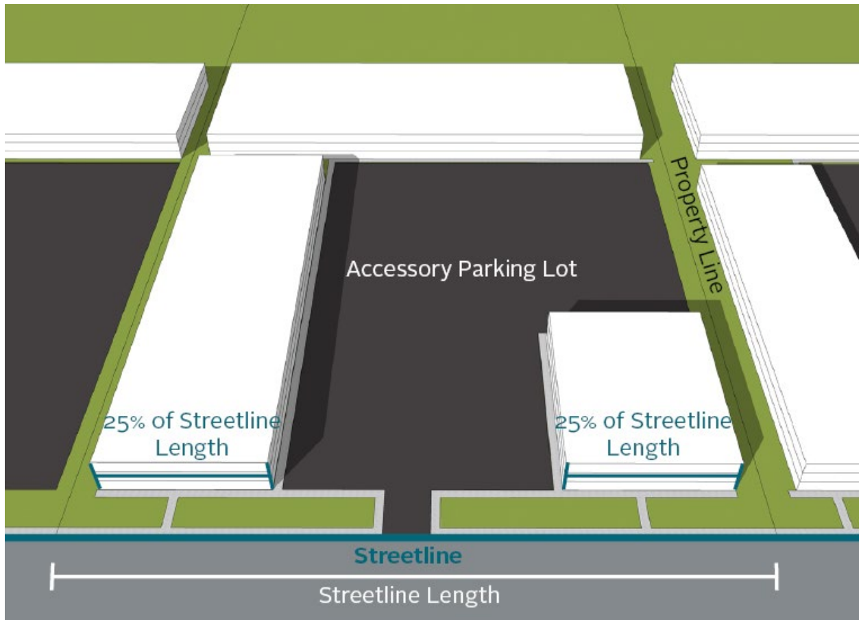
Diagram PG-15: Streetwalls without parking between the streetline and the streetwall extend for a combined 50% of the total streetline length, per Clause PG-205(2)(b)
