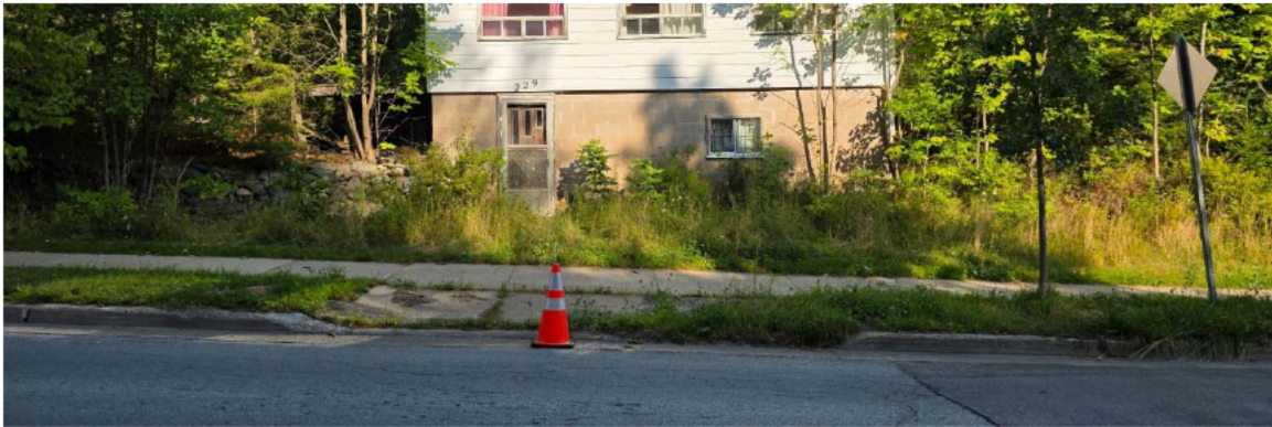
Exhibit 2.5 – Pylon used for Stopping Sight Distance Field Measurements
