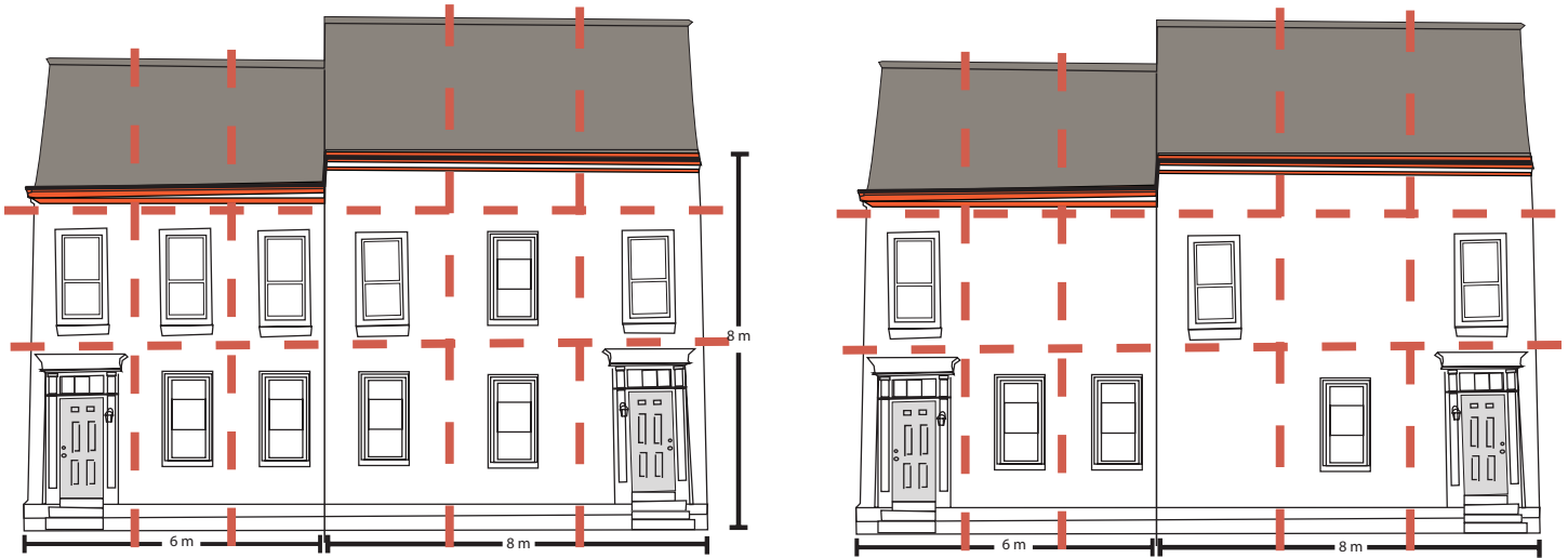
Front façades showing variable appropriate widths, including three bays each, and a cornice line of less than 8m in height. Both images show windows which are taller than wide. The image on the right demonstrates one possible fenestration pattern which satisfies only the minimum requirement of one window within each bay and storey.
