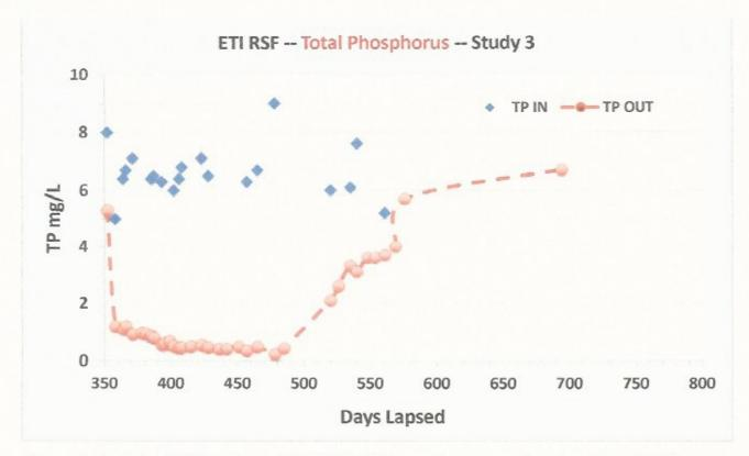
Figure 3. Study 3 of RSF testing at MASSTC; EC-P was disconnected on Day 491 and RSF effluent returned to background levels close to sewage levels.
