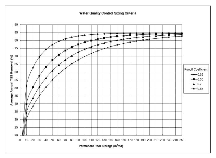
Figure 5-1 Example of Sizing Permanent Pool Storage for Water Quality Control
