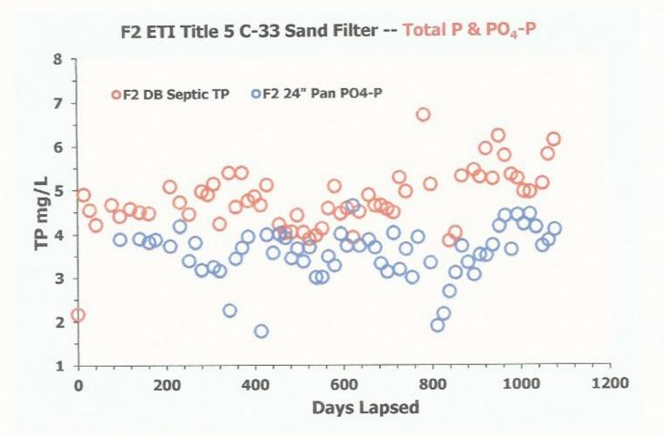
Figure 5. Results of MASSTC Site F2 for C-33 Sand Filter in 1999 – 2002. Removal of TP between septic tank effluent and soil percolate is 20 – 25%
