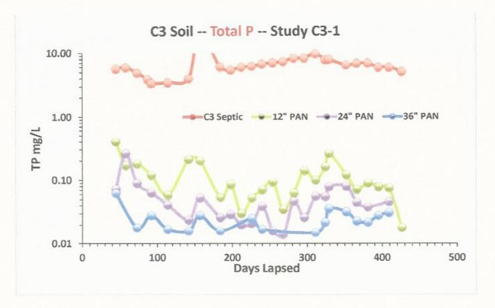
Figure 4. On-going EC-P Study C3-1 for P removal in septic tank + soil leach field. High percentages of P removal are attained and generally improve with time.
