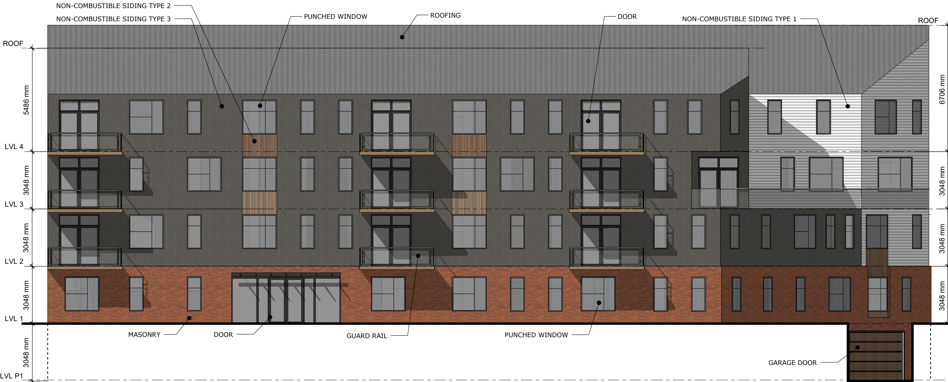
MULTI - NORTH EAST ELEVATION
