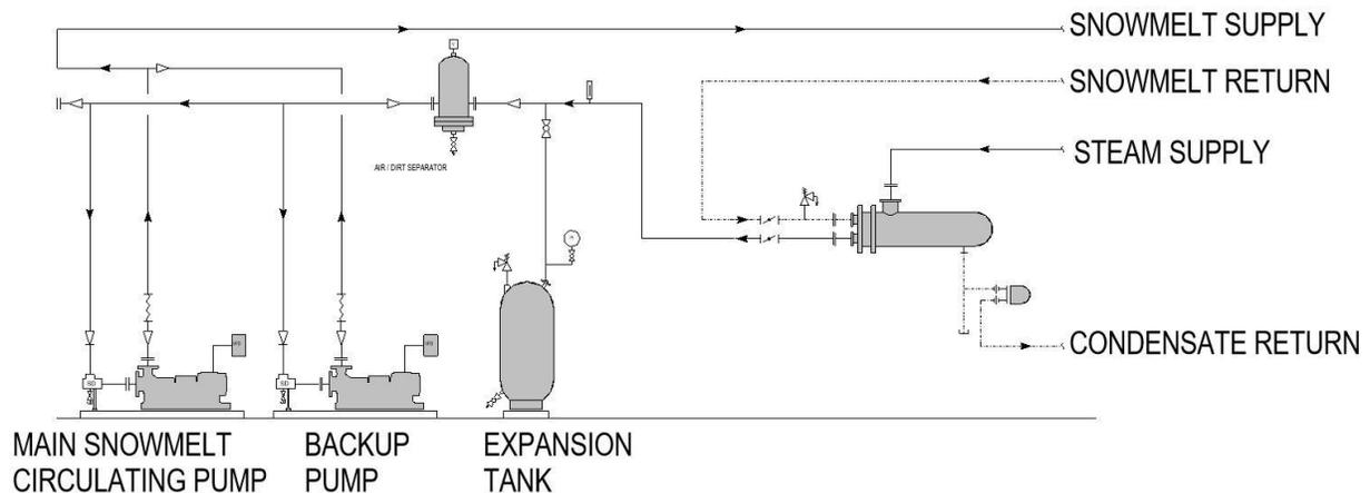
Snowmelt system schematic using steam from MSVU Heating Plant.
