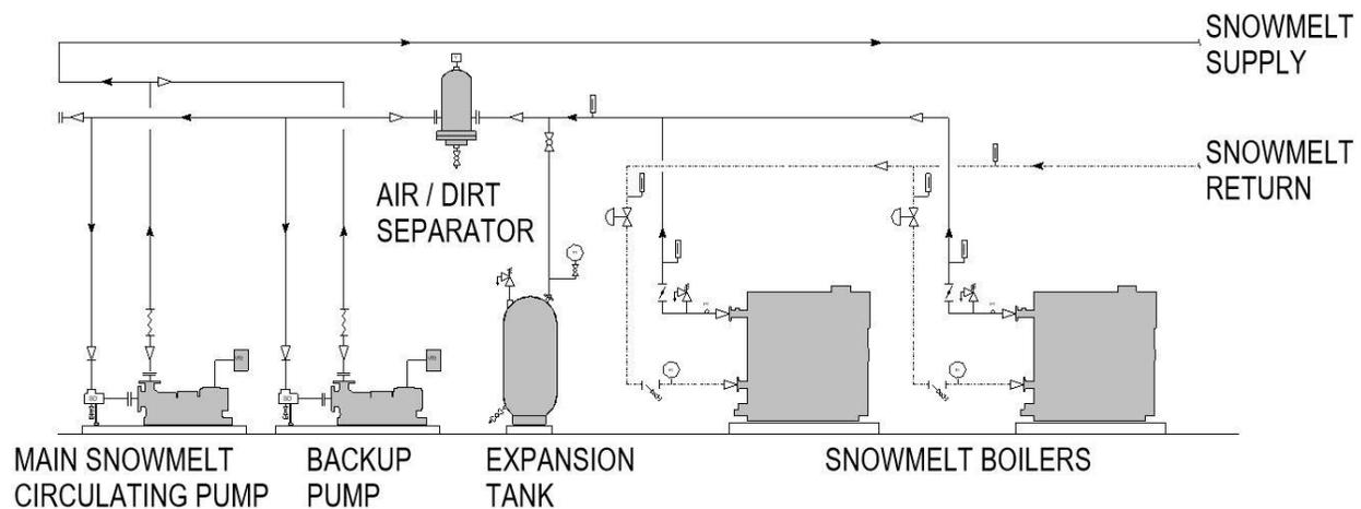
Snowmelt system schematic using dedicated boilers
