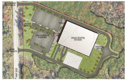
The site can accommodate up to about 238 parking spaces located between the building and Prospect Road and includes loading bays at the rear of the building supported by a truck access roadway along the periphery of the site. Access points, internal circulation, and turning areas should be deigned to accommodate these larger vehicles. The above figure shows a conceptual layout well suited to accommodate these truck movements with minimal impact to on-site circulation of regular day traffic.
