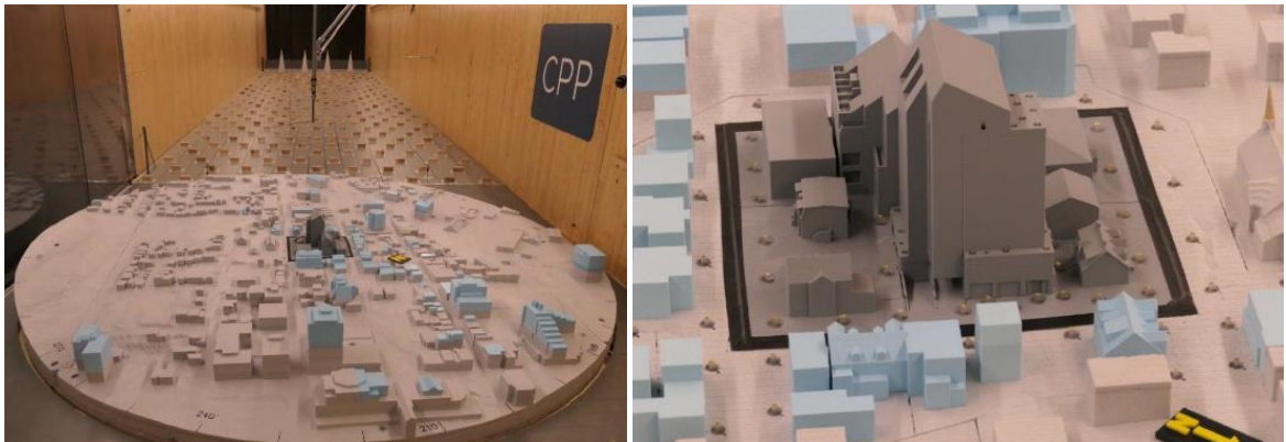
Figure 1: Photographs of Wind Tunnel Model in a CPP Boundary Layer Wind Tunnel
