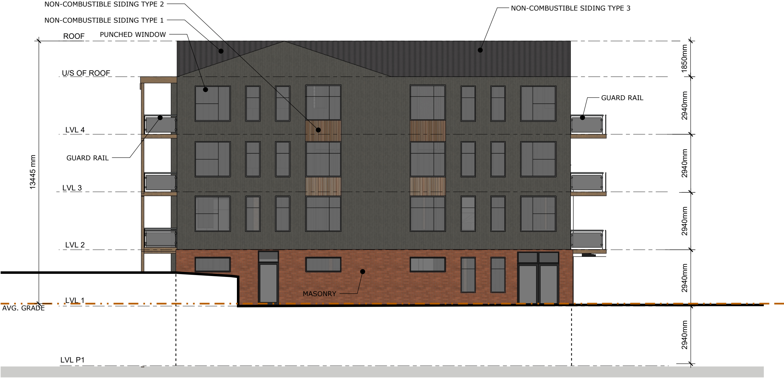
MULTI - SOUTH EAST ELEVATION
