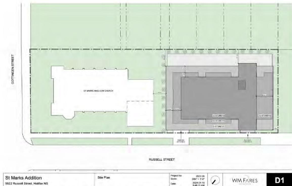
Figure 43: Revised Site Plan, April 2024, illustrating setbacks and stepped back upper floors.
