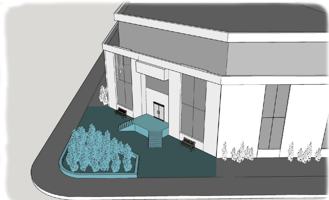
Diagram 13: Eroded building corner, per Subclause 361(b)(v)
