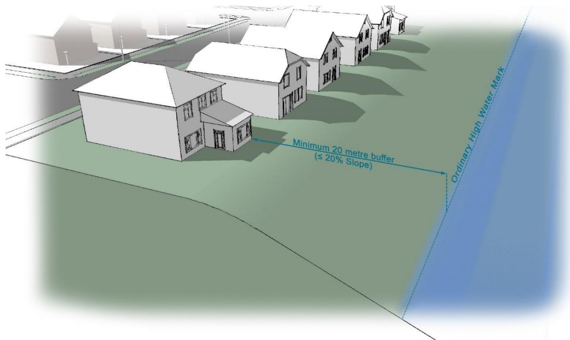
Diagram 3: Minimum required watercourse buffer, per Subsection 75(2)
