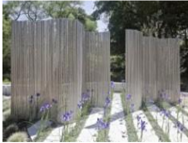
Diagram A1-5: Examples of smaller-scale building elements and soft landscaping features for wind control.
