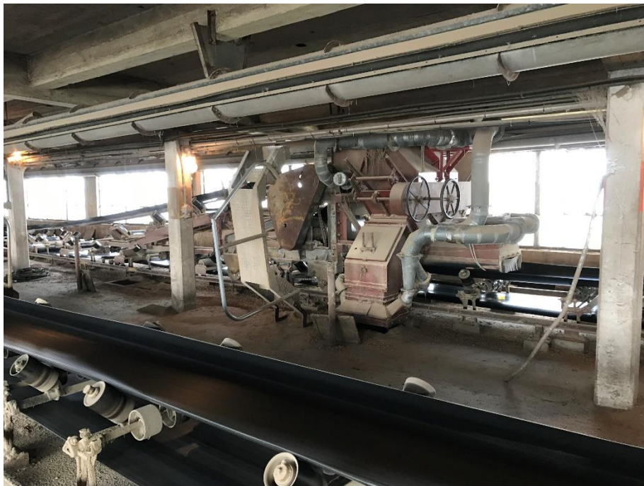
D.18: Belt tripper in Annex 2.
