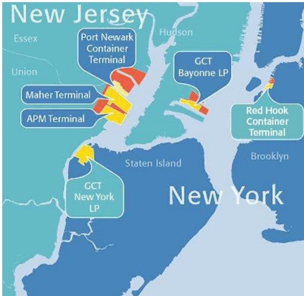
Red Hook Terminals operates the only terminal handling containers on the eastern side of the harbor. Red Hook Terminals is a multi-product terminal, capable of bulk and breakbulk cargoes, containers, yachts, heavy lifts, autos, or special project cargoes. The Red Hook terminal cannot handle large container ships due to draft limitations (42 ft). The company also operates a barge terminal in Newark, New Jersey and a cross-harbor rail barge.<sup>67</sup>
