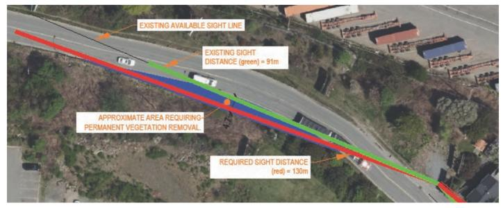
Field measurements show that the available sight distances based on existing vegetation is about 91 meters (GREEN LINE) with a required sight distance of 130 meters (RED LINE). This results in an area requiring permanent vegetation removal along the south side of the roadway as shown be the BLUE shaded area.
