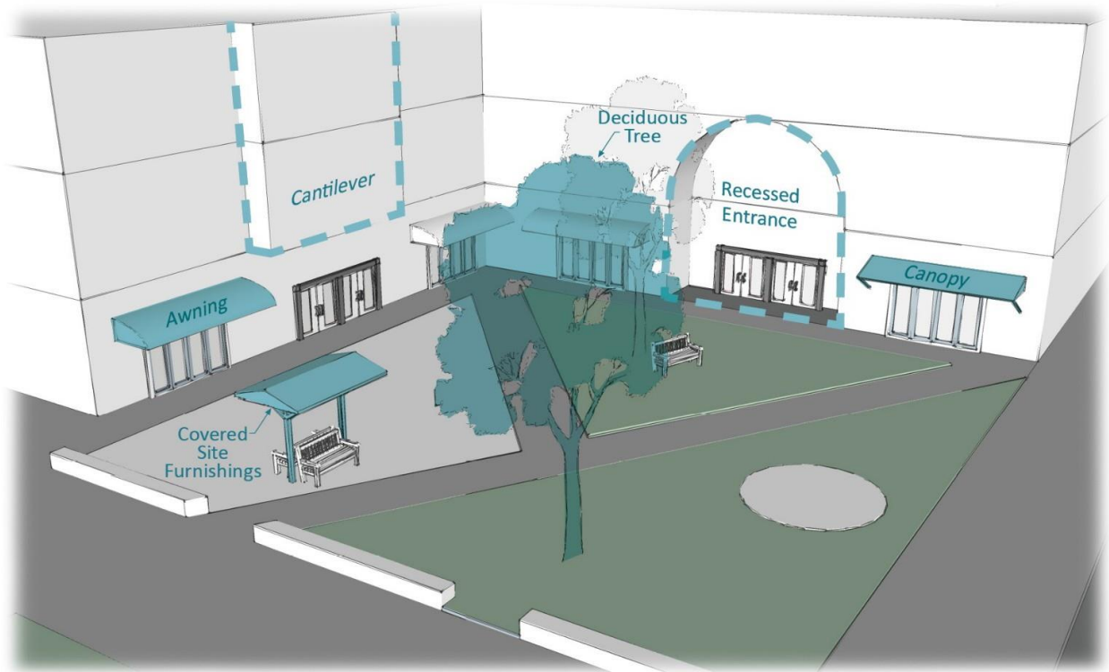
Diagram 10: Weather protection for outdoor amenity space, per Clause 356(2)(b)
