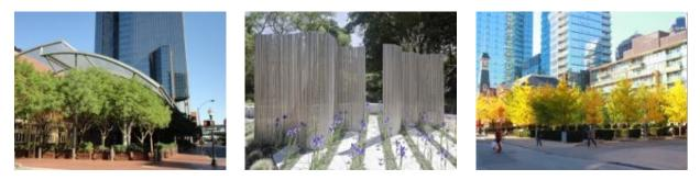
**Diagram PGA1-5**: Examples of smaller-scale building elements and soft landscaping features for wind control.
