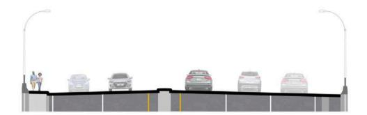
There are no designated cycling facilities on Grahams Grove, cyclists must dismount and use the sidewalk in this high traffic area. The pedestrian sidewalk is narrow and not protected by a barrier.
