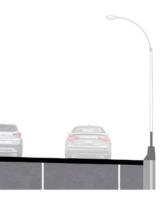
A protected multi-use path would create space for cyclists and pedestrians to move safely across the Braemar overpass separately from cars. Accommodating space for this would result in narrower lanes and lower speed limits for vehicle traffic.
