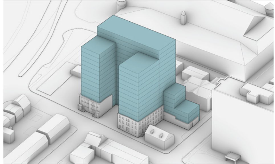
Alternative 3: Conserve building facades. Remove and replace interiors. Construct new building(s) within existing footprints.
