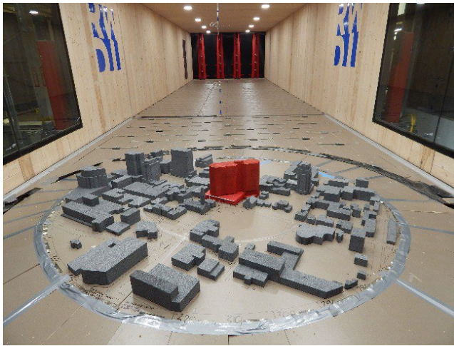
Diagram A1-2b: Photo of modelled buildings in a boundary-layer wind tunnel
