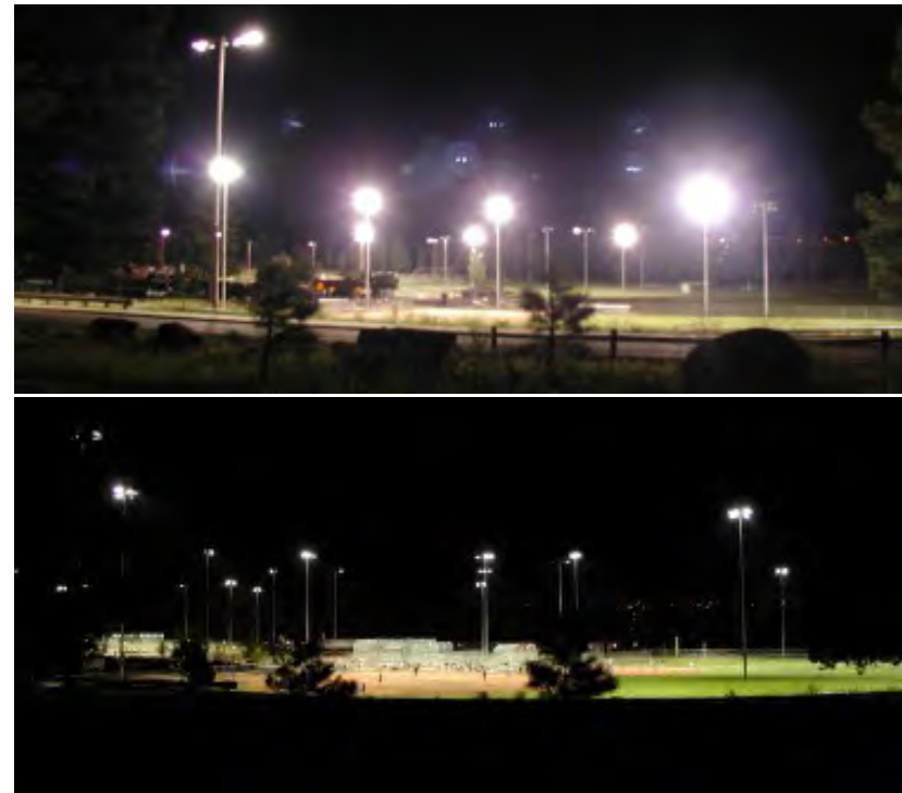
Figure 29: Lighting for sport uses can be intrusive within communities. This image illustrates the difference between shielded and unshielded sport lighting (Flagstaff Dark Skies Coalition, 2014).
