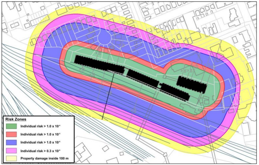
Figure V: Site plan showing risk zones for restricted (green), low-density residential (red), high-density residential (blue), and sensitive (pink) land uses and the area with potential for significant property damage.
