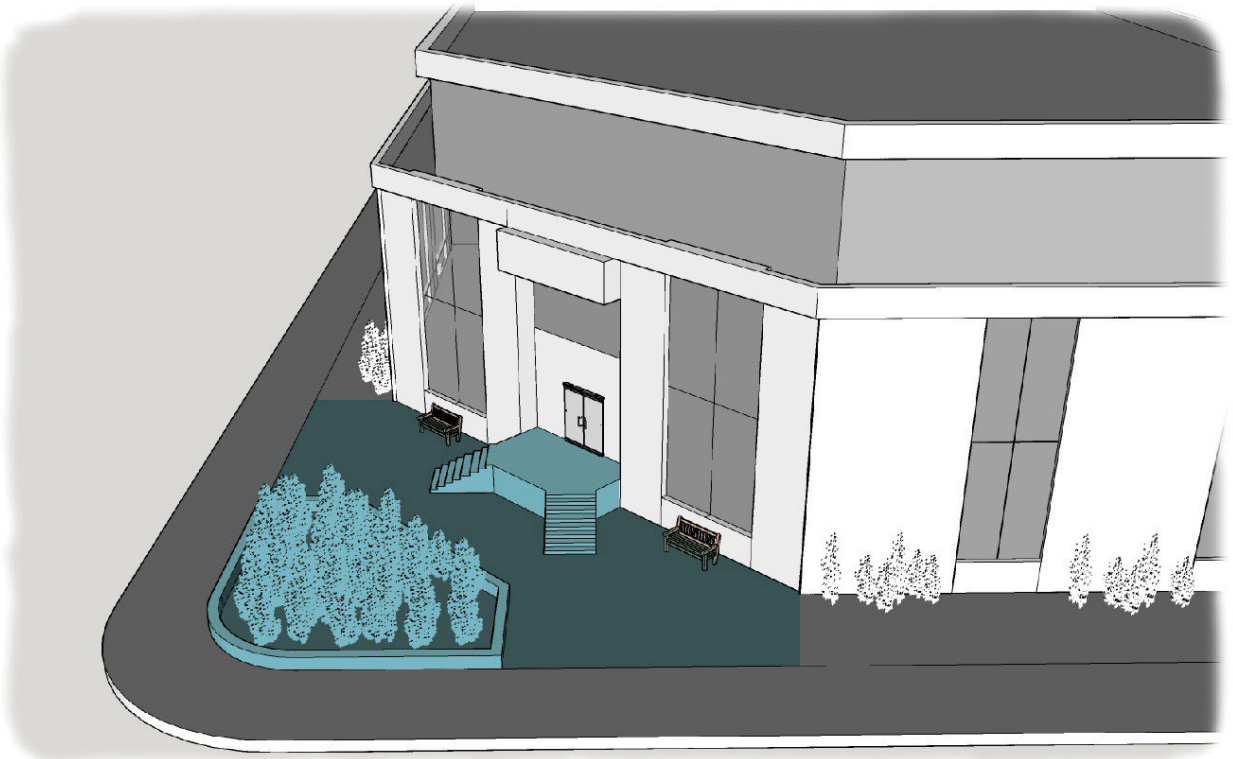
Diagram 13: Eroded building corner, per Subclause 361(b)(v)
