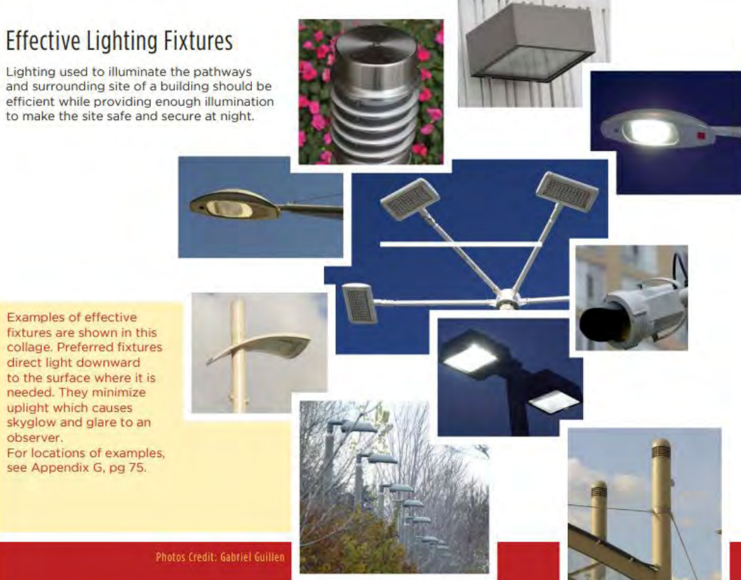
Figure B2: Effective Lighting Fixtures that cast downward light to illuminate pathways while reducing light trespass and glare (City of Toronto, 2017).
