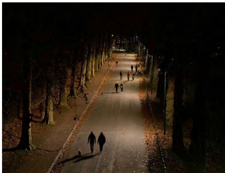
Figure 7: The City of Lille, France, has implemented a 'nocturnal corridor' using an amber colour temperature (i.e., 2,200K - 2,700K). This limits disruption to wildlife while still allowing for evening and early morning recreation (Schröder, 2023).
