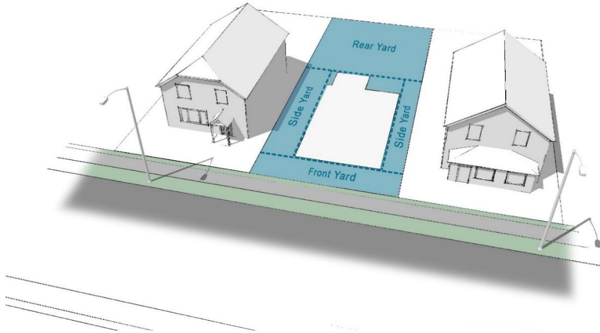
Diagram PG-27: Front yard, side yard, and rear yard, per Subsections PG-238(87), PG-238(185), and PG-238(213)
