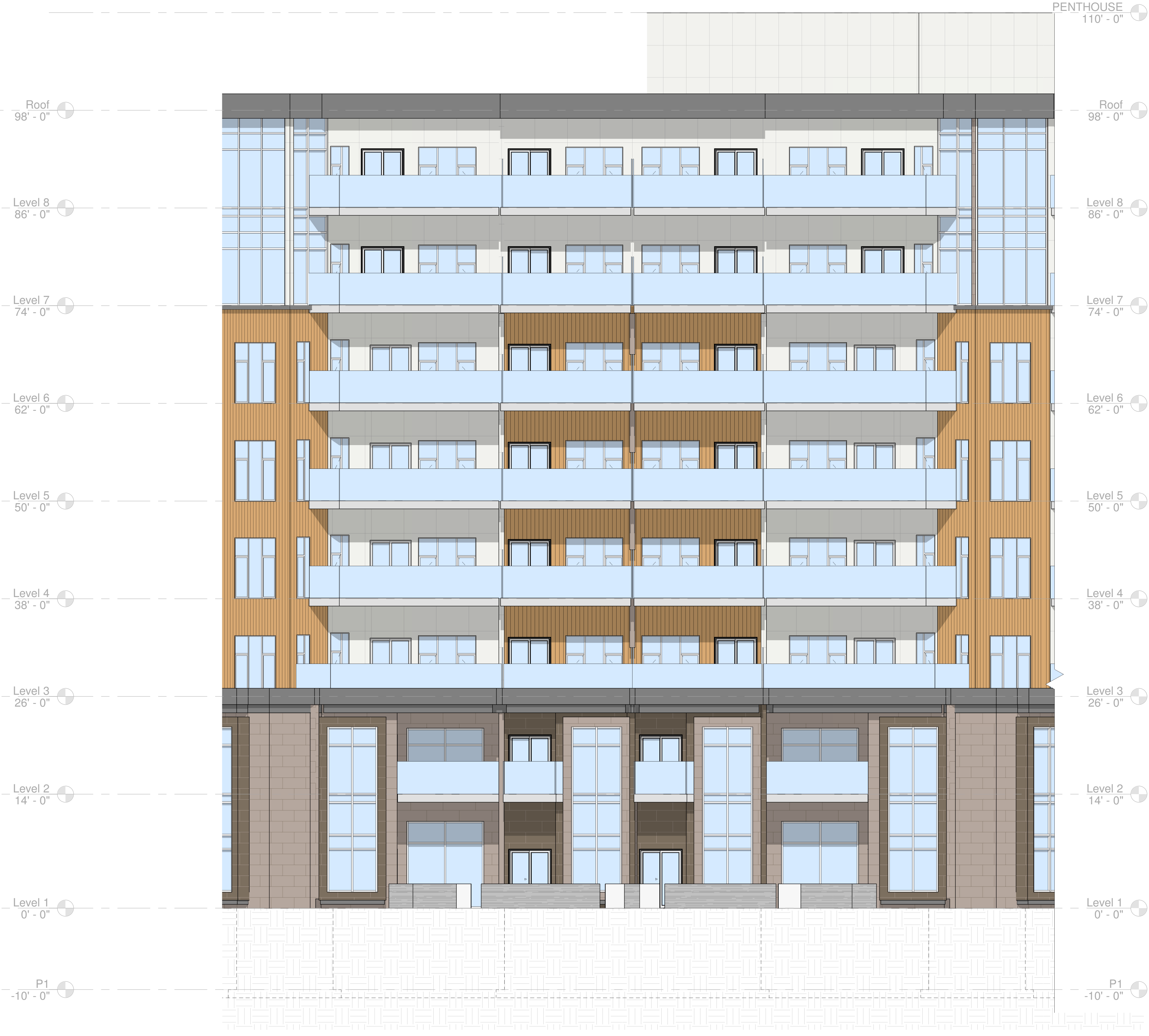
② North-West Elevation 1/8" = 1'-0"
