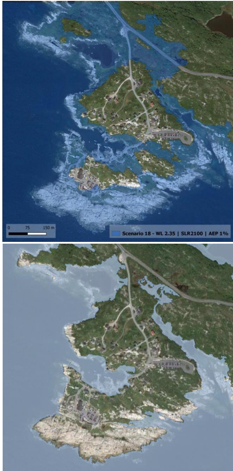
Figure 5-15: Comparison of flood extents developed for Peggy's Cove (100-year return period, current climate conditions). CBCL, 2020b (top, including wave run-up) and present study (bottom, static storm surge excluding wave run-up).
