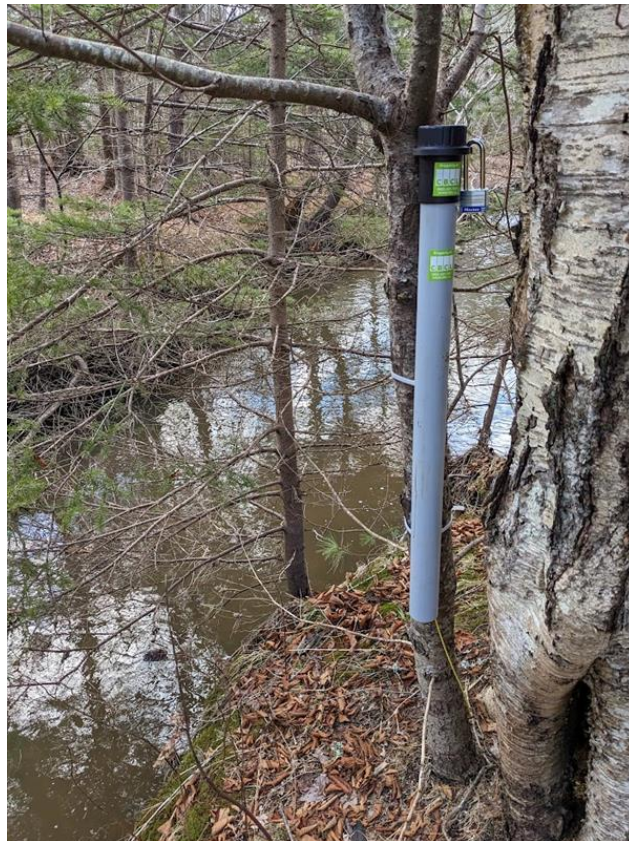
Figure 11-1: Field installation of the Solinst Levelsender telemetry unit at Bissett Creek, fastened to the tree with plastic tie straps. The Levelogger unit is deployed within the adjacent watercourse.
