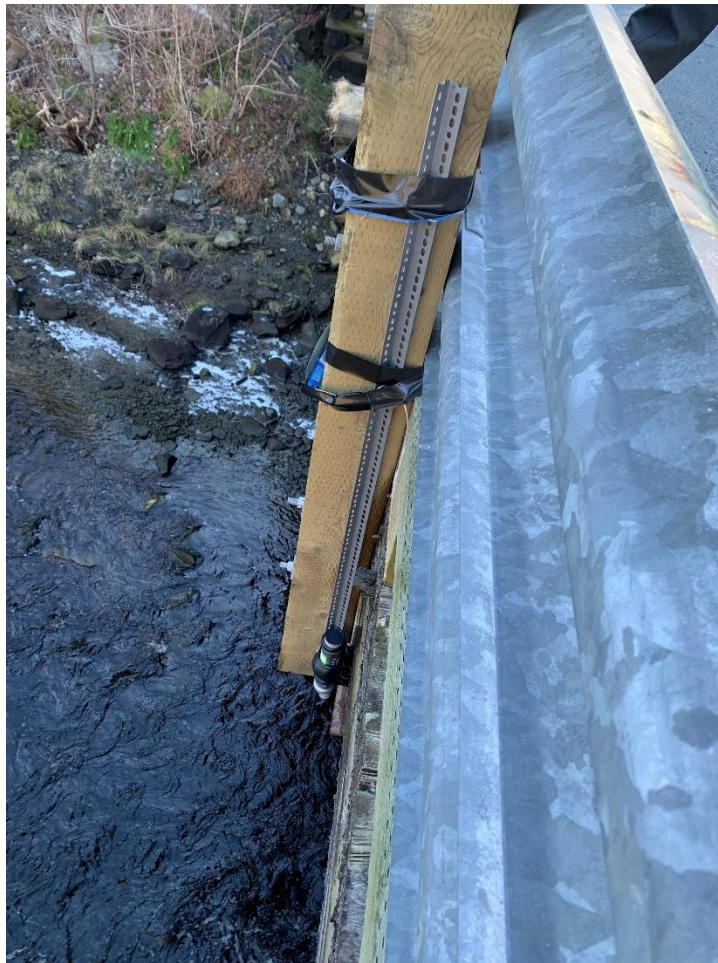
Figure 11-9: Deployment location at West Side Road bridge. The ToltHawk instrument itself can be seen at the bottom of the guardrail post.
