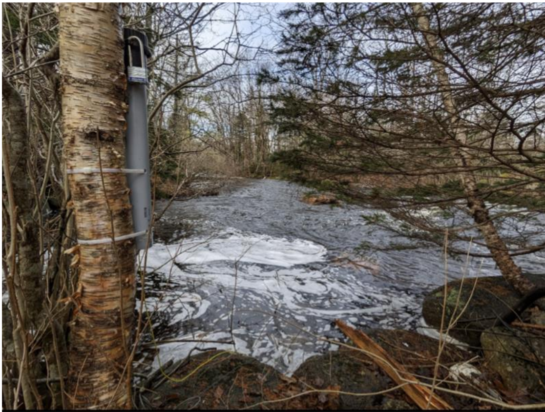
Figure 11-3: Field installation of the Solinst Levelsender telemetry unit at East River (Tantallon), fastened to the tree with plastic tie straps. The Levelogger unit is deployed within the adjacent watercourse.
