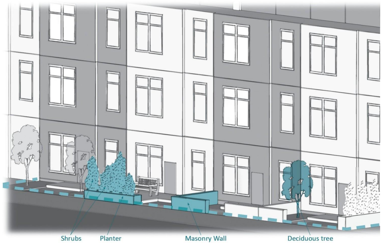
Diagram PG-9: Methods for providing privacy to grade-related dwelling units, per Section PG-165
