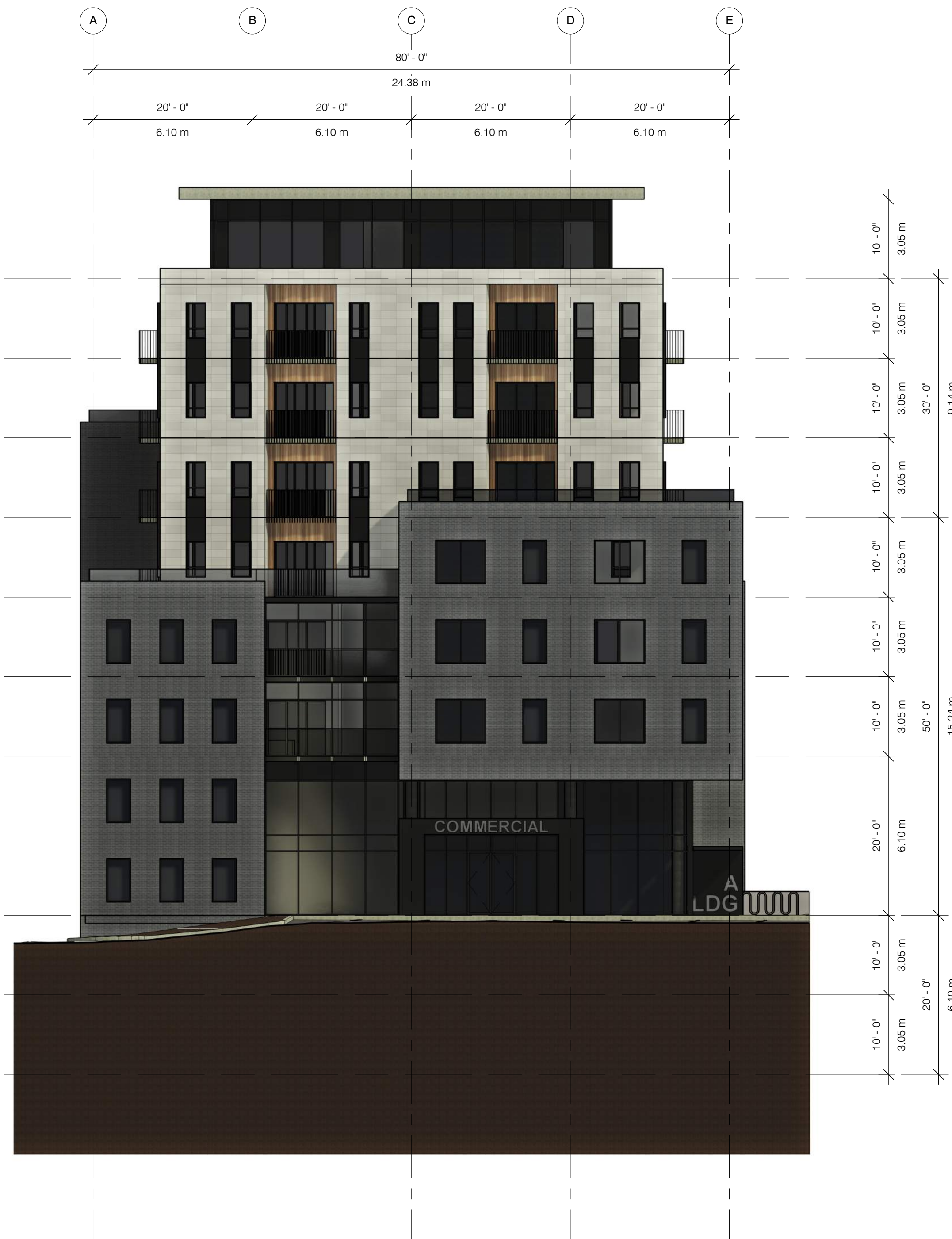
1 Building A - North Elevation A302 3/32" = 1'-0"
