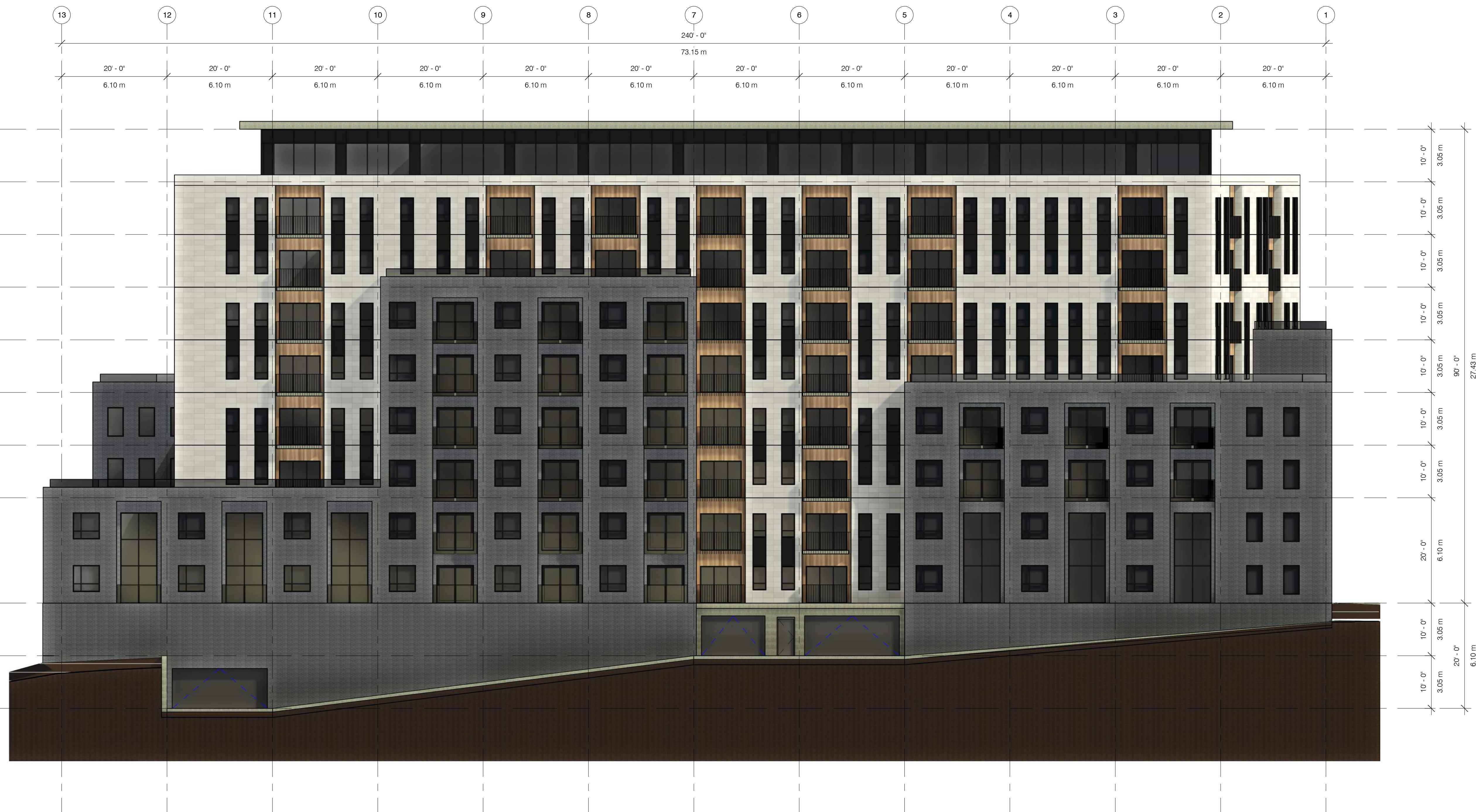
1 Building A - East Elevation A301 3/32" = 1'-0"
