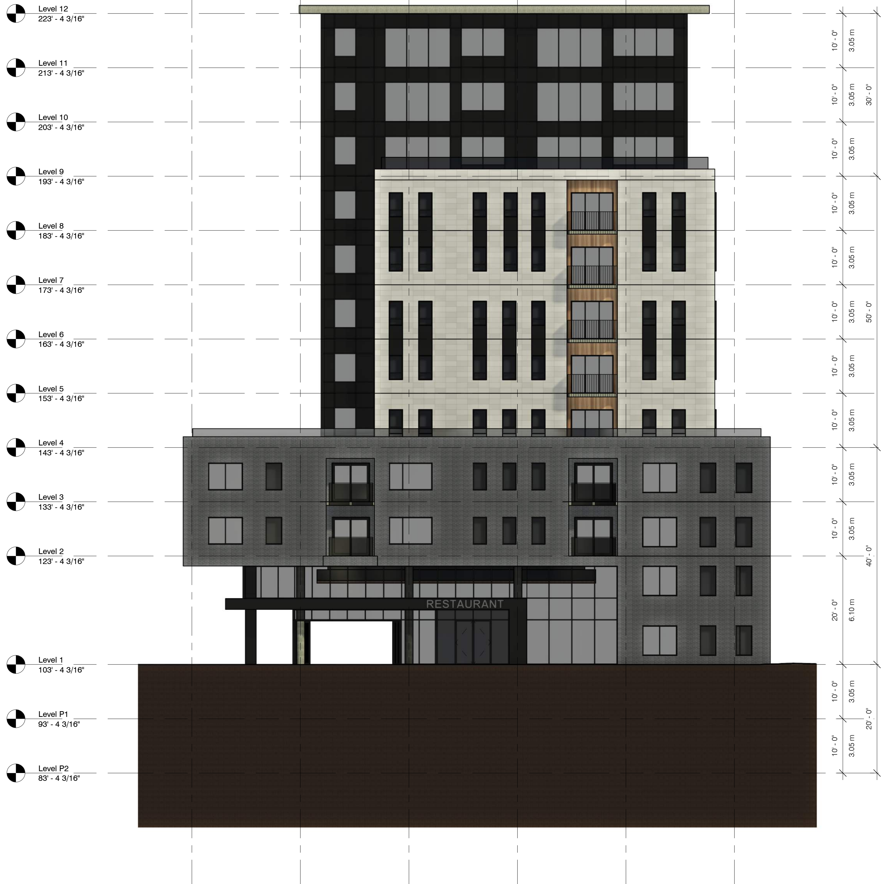
1 Building B - North Elevation 3/32" = 1'-0"
