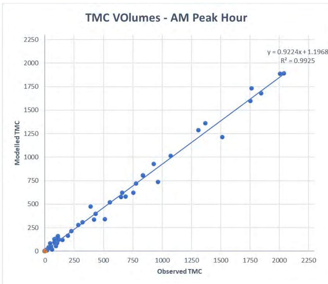
**Figure 3-3: Turn Volume Calibration – AM Peak Hour**
