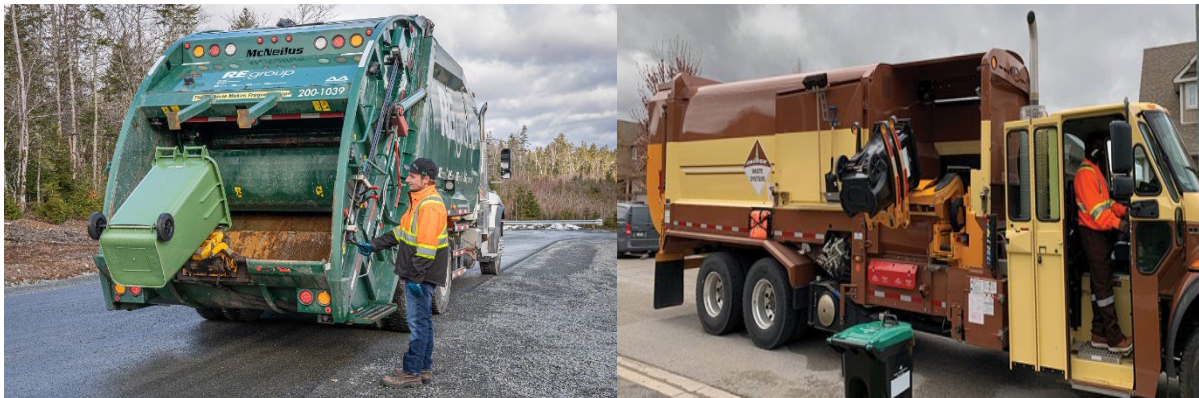
Figure 1 – Semi-Automated Collection (Left) Source: REGroup and Automated Collection (Right) Source: The Creemore Echo
