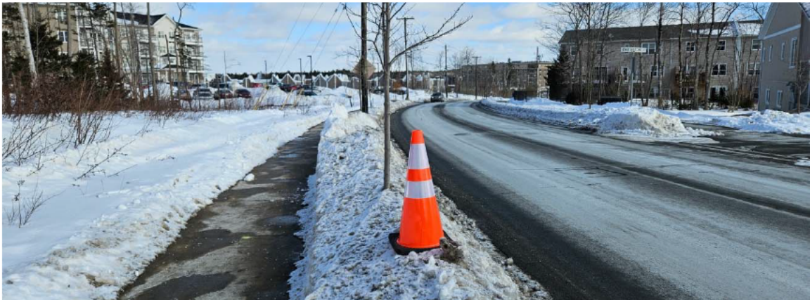
Exhibit 2.8 – Pylon used for Stopping Sight Distance Field Measurements
