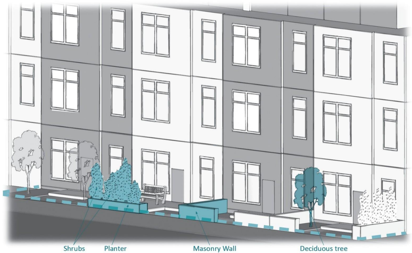
Diagram PG-8: Methods for providing privacy to grade-related dwelling units, per Section PG-152
