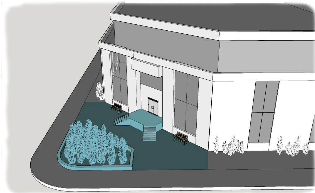
Diagram PG-10: Eroded building corner, per Subclause PG-155(b)(v)
