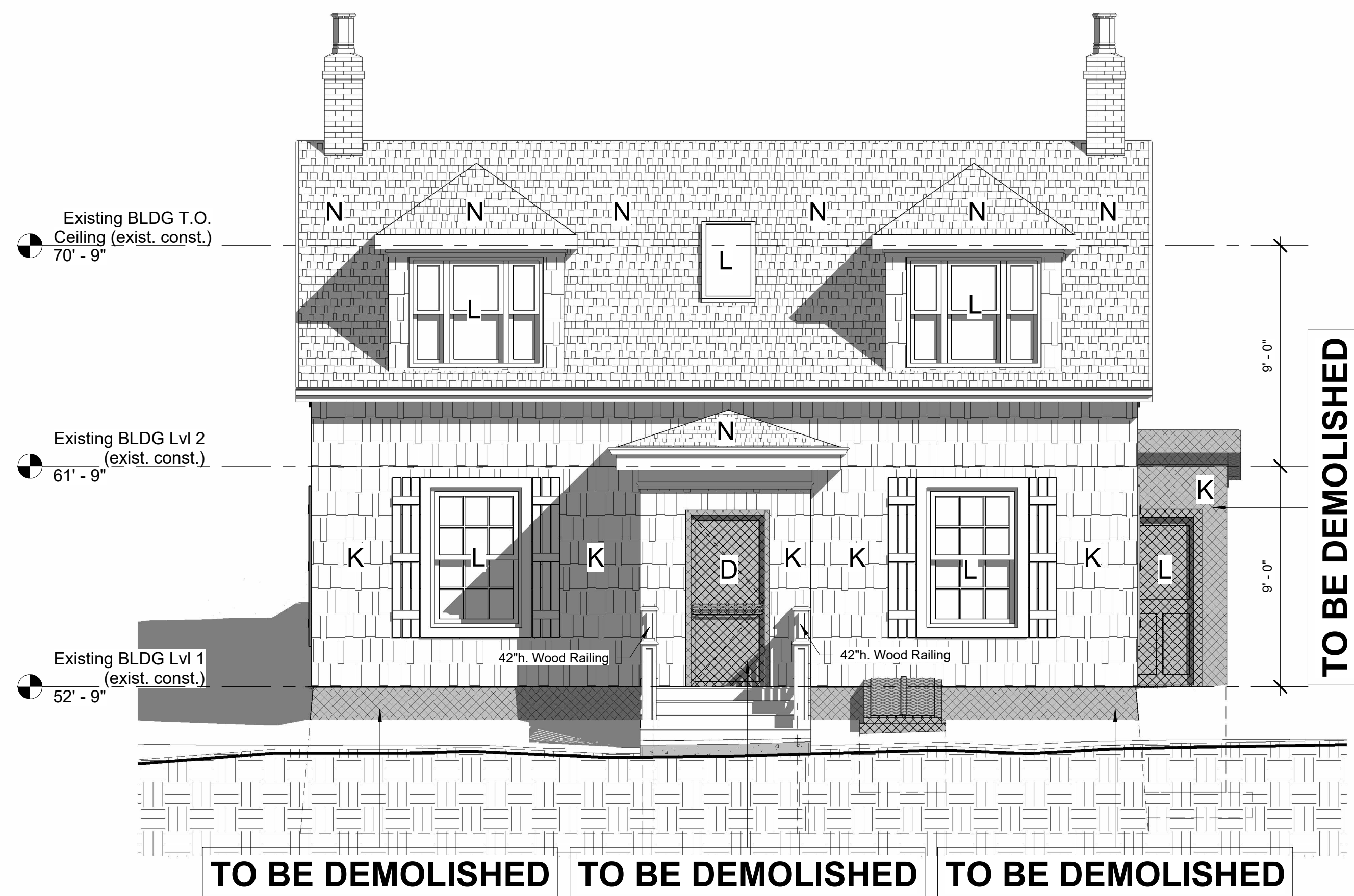
③ Honeycote - South (existing const.) 1/4" = 1'-0"
