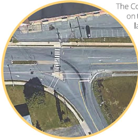
The Cole Harbour Road intersection with Bissett Road is a 3-leg tee intersection on the south side of Cole Harbour Road. It is characterized by a single through lane in each direction on Cole Harbour Road along with a dedicated left turn lane in the westbound direction. The two through lanes in the eastbound direction terminate with a dedicated right turn channelized movement to Bissett Road and a single through lane eastbound on Cole Harbour Road.
