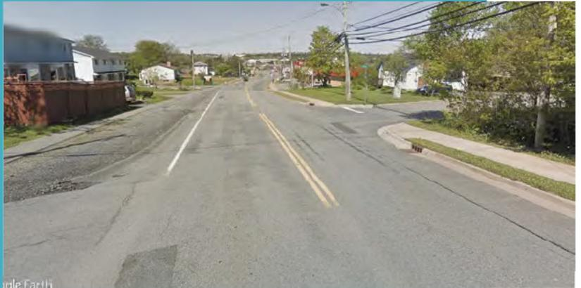
**Cole Harbour Road (East of Bissett Road)** has a two-lane undivided cross section with concrete curb and gutter on the north side of the street and a variation of asphalt and concrete sidewalks and gravel shoulders on the south side.
