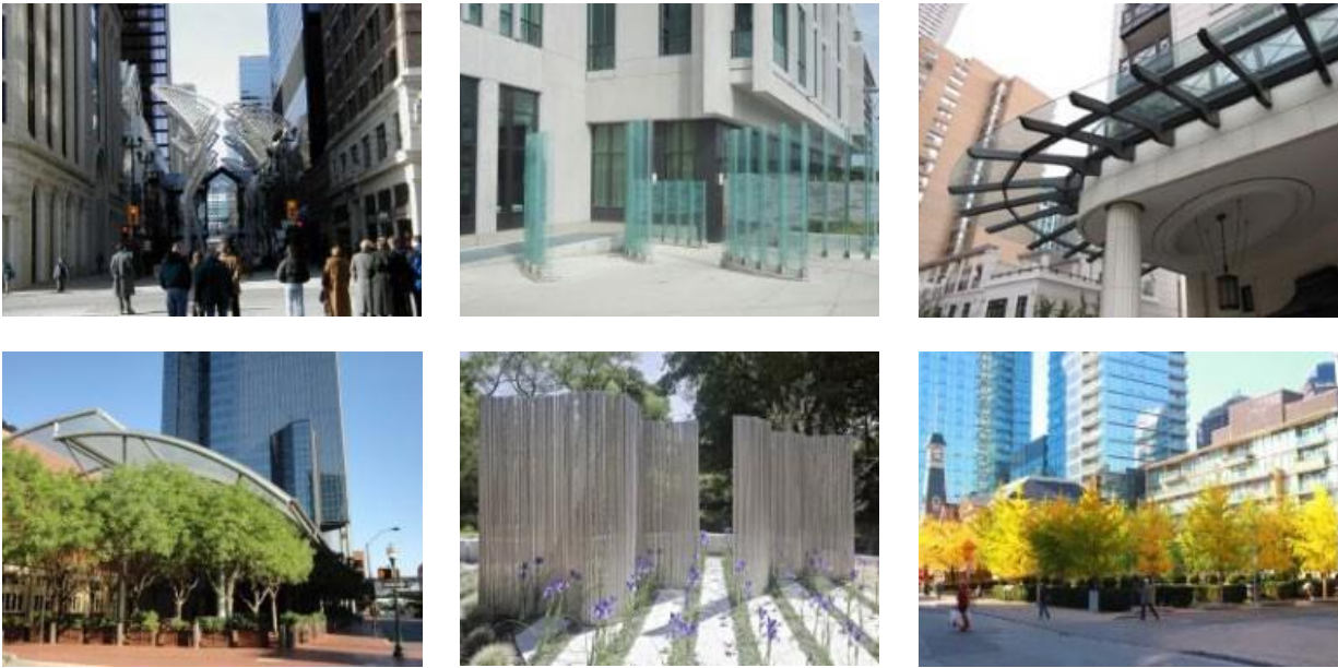
Diagram A1-5: Examples of smaller-scale building elements and soft landscaping features for wind control.
