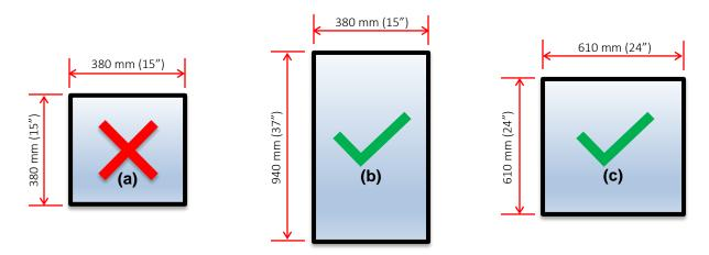
**Window (a)** has an openable portion that is 380 mm x 380 mm (15" x 15"). While this meets to the width and height requirements for unobstructed opening's, it does not meet to the area requirements as the opening is only  $0.144 \, \text{m}^2$  (255 Sq. in.) in area.
