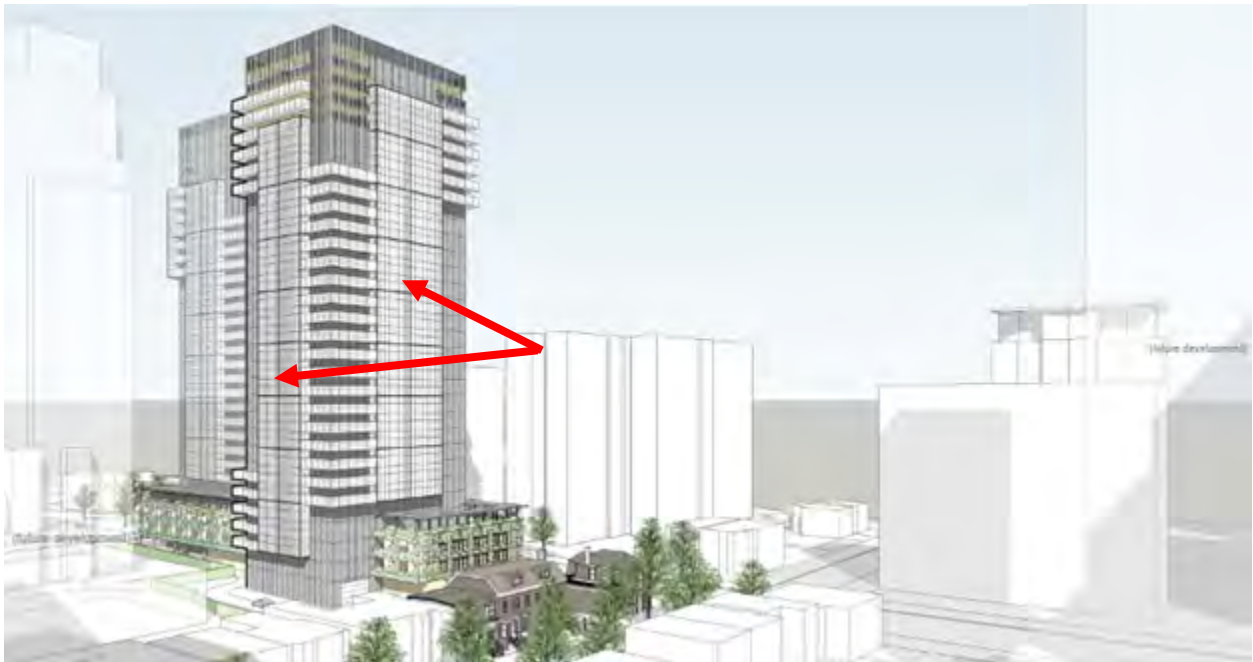
Figure 4: Signature architectural projections identified by red arrows
