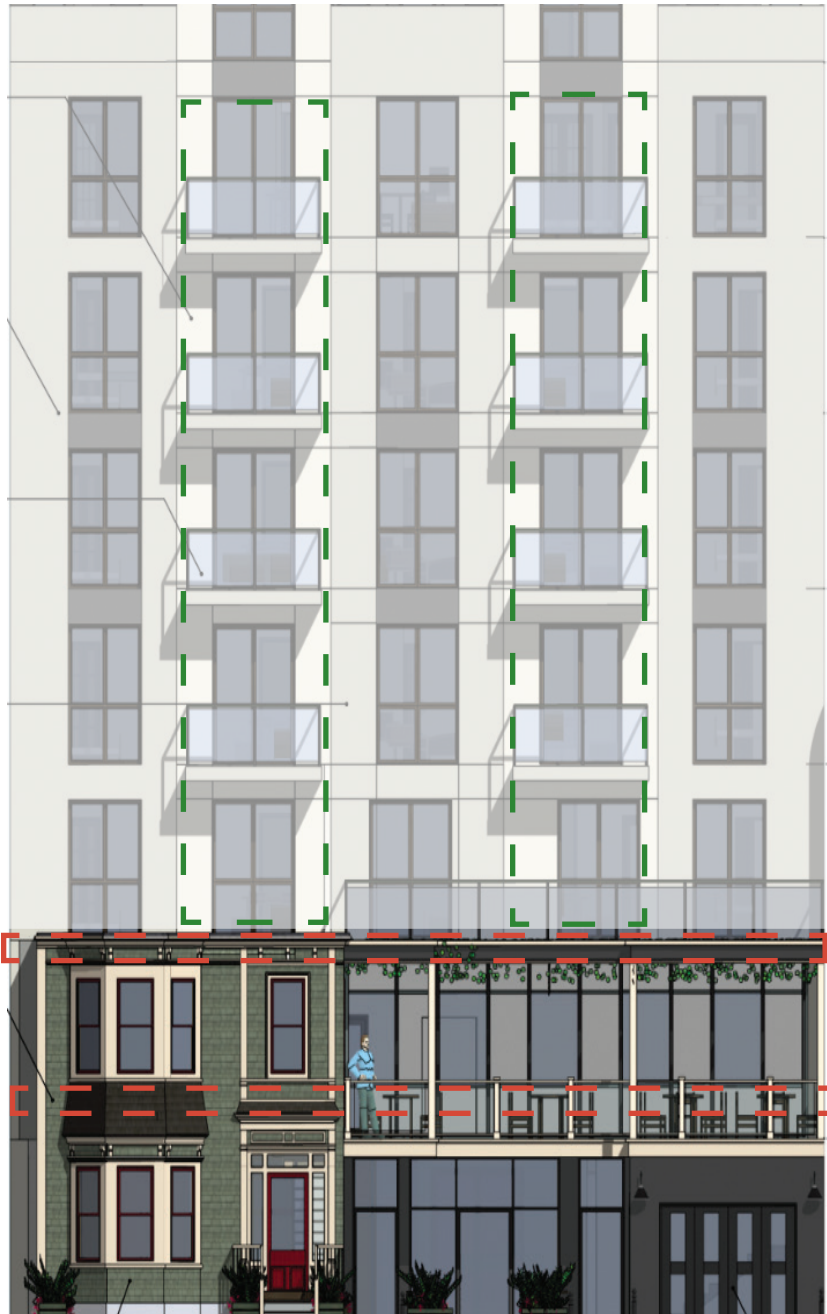
Fig. 15 Vertical and Horizontal Elements characteristics of the Halifax Box style extended in new facade
