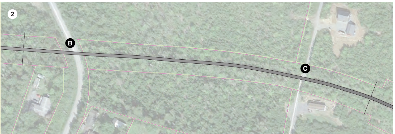
B | Crossing at Brian Dickie Drive: Install standard trail crossing signage on road and trail (WC-46R / WC-7S, RA-1, RB-93), and install boulders or gate to restrict motorized access
