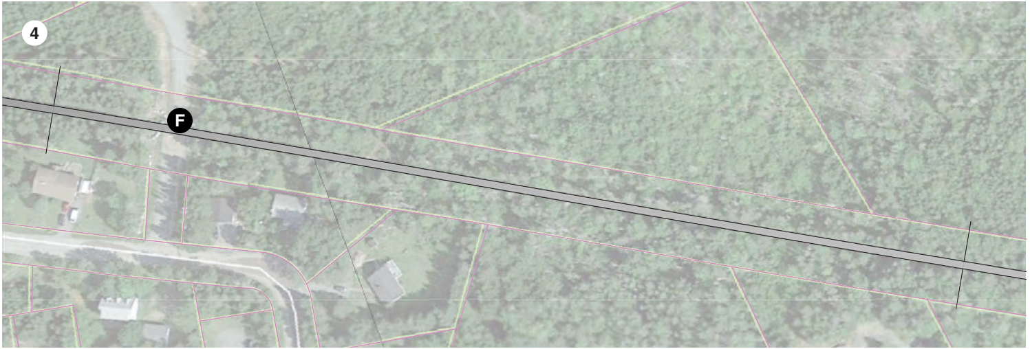
F | Crossing at Darius Lane: Install standard trail crossing signage on road and trail (WC-46R / WC-7S, RA-1, RB-93), and install boulders or gate to restrict motorized access
